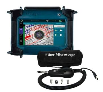
The optional fiber optic microscope can be used to quickly and easily check the connector end faces and provide an automatic "pass/fail" assessment
