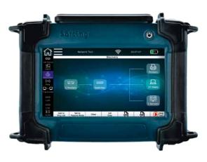
For network discovery, simply connect NetXpert XG to a switch (copper and WiFi included in base unit, fiber if enabled)
